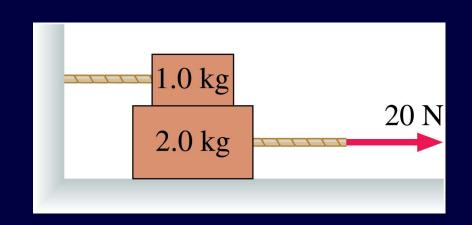
7.24: The 1.0 kg block in the figure is tied to the wall with a rope. It sits on top of the 2.0 kg block. The lower block is pulled to the right with a tension force of 20 N. The coefficient of kinetic friction at both the lower and upper surfaces of the 2.0 kg block is  $\mu k = 0.41$ . What is the tension in the rope holding the 1.0 kg block to the wall? What is the acceleration of the 2.0 kg block?
