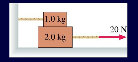
7.24: The 1.0 kg block in the figure is tied to the wall with a rope. It sits on top of the 2.0 kg block. The lower block is pulled to the right with a tension force of 20 N. The coefficient of kinetic friction at both the lower and upper surfaces of the 2.0 kg block is  $\mu k = 0.41$ . What is the tension in the rope holding the 1.0 kg block to the wall? What is the acceleration of the 2.0 kg block?
