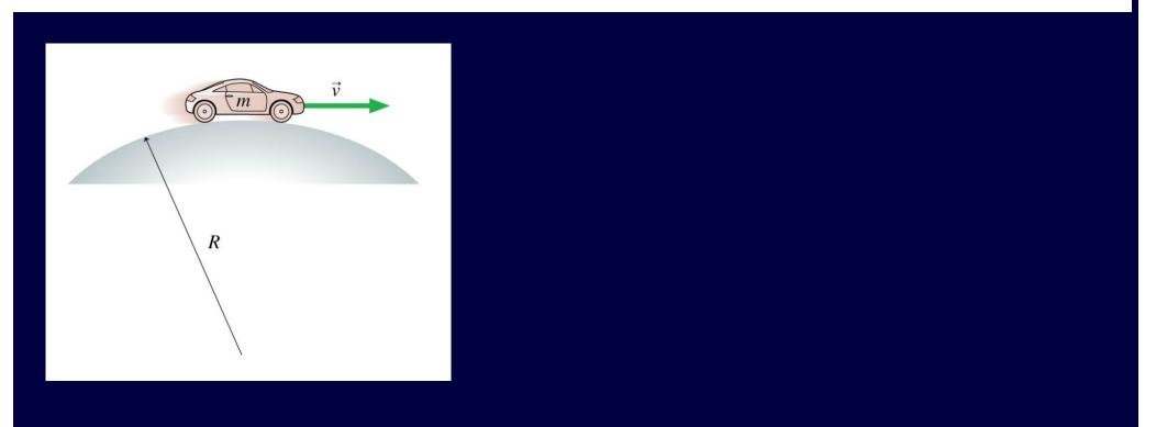
A car of mass m = 1000 kg drives over a hilltop that has a radius of curvature R = 0.120 km travelling at a constant speed of 20 m/s as in the figure below. (a) At this speed, what is the normal force that the ground applies to the car at the very top of the hilltop, as pictured? (b) At what speed would the car be traveling when its tires just barely lose contact with the road when the car is at the top of the hilltop?
