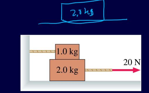
7.24: The 1.0 kg block in the figure is tied to the wall with a rope. It sits on top of the 2.0 kg block. The lower block is pulled to the right with a tension force of 20 N. The coefficient of kinetic friction at both the lower and upper surfaces of the 2.0 kg block is  $\mu k = 0.41$ . What is the tension in the rope holding the 1.0 kg block to the wall? What is the acceleration of the 2.0 kg block?
