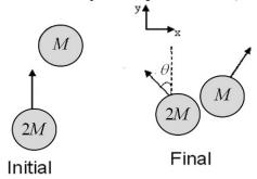
After the collision, the disk with mass 2M is deflected  $\theta = 15.0^{\circ}$  and has speed 3.00 m/s as shown in the figure.
