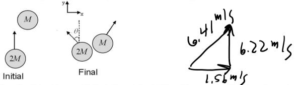
After the collision, the disk with mass 2M is deflected  $\theta = 15.0^{\circ}$  and has speed 3.00 m/s as shown in the figure.
