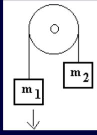
Two blocks,  $m_1 = 5$  kg and  $m_2 = 3$  kg, are connected by a massless rope around a frictionless, massless pulley as pictured below. Which equation below would be a result of applying Newton's second law correctly to either block 1 or block 2? Call the tension acting on block 1  $T_1$  and the tension acting on block 2  $T_2$ .
