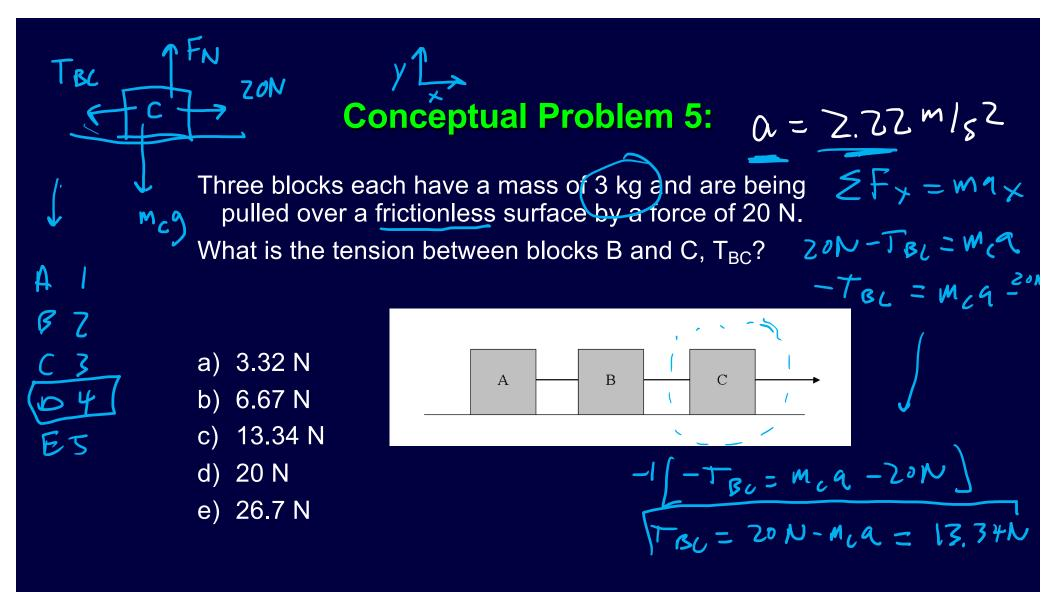
Three blocks each have a mass of 3 kg and are being pulled over a frictionless surface by a force of 20 N.What is the tension between blocks set of 20 M.
