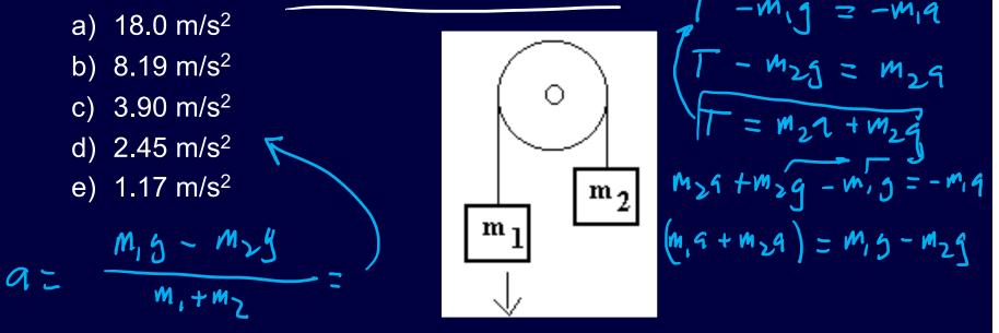
Two blocks,  $m_1 = 5$  kg and  $m_2 = 3$  kg, are connected by a massless rope around a frictionless pulley as pictured below. What is the acceleration of block 1?
