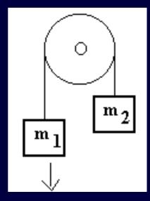
Two blocks,  $m_1 = 5$  kg and  $m_2 = 3$  kg, are connected by a massless rope around a frictionless, massless pulley as pictured below. What is the acceleration of block 1?
