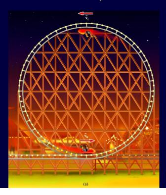
What is the minimum speed you must have at the top of the roller coaster loop to keep the wheels on the track? The loop has a diameter of 20m.
