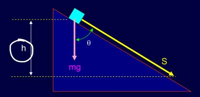
Gravity does zero work for motion in the x-direction
