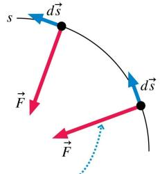
The force is everywhere perpendicular to the displacement, so it does no work.
