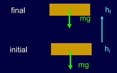
By moving the block up a distance h, it gains potential energy of mgh!
